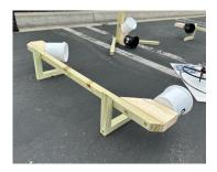
Wall Base - 1 4x4x100cm(2x2x42in), 4 4x4x50cm(2x2x21in) w/ 45-degree angle cut both ends 2 Linear Rails
