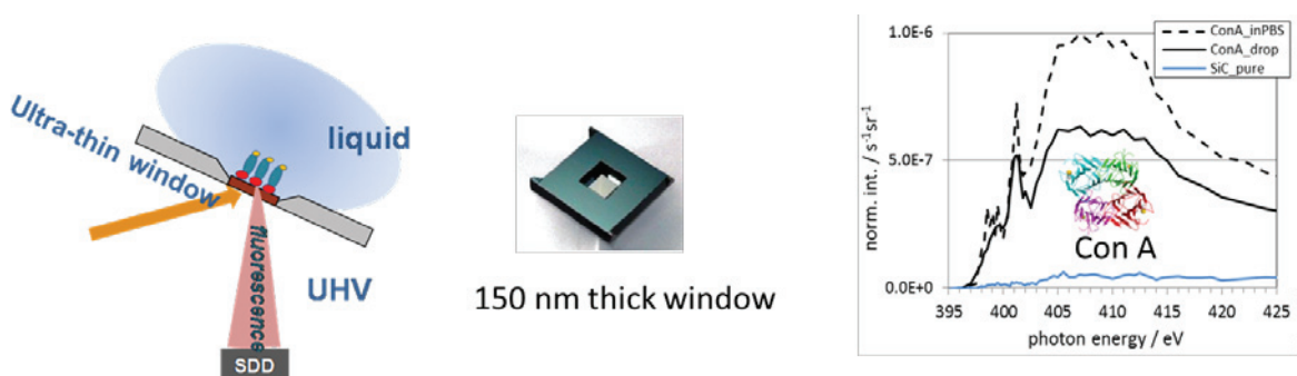
FIGURE 2. The left part shows the experimental setup using a thin window functionalized on one side. The right figure shows the N K – NEXAFS of the blank window and the NEXAFS with Concanavallin A in solution and attached to the functionalized surface of the window.
