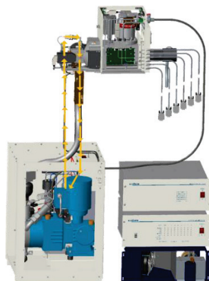
FIGURE 2. A complete MetalJet X-ray source with source head, pump box, support electronics and water-chiller.).
