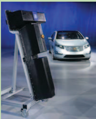
This T-shaped battery, a replica of the battery used in the Chevy Volt, includes Argonne cathode technology. LG Chem licensed the materials and created the battery. Image courtesy General Motors.
