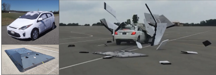
GVT (top left) over the LPRV, LPRV (bottom left), and car impacts GVT at 25 mph (right), Source: NHTSA
