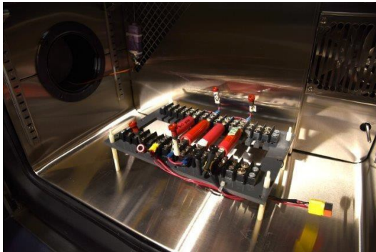
The Impedance Measurement Box can assess a single battery cell or battery strings, which are commonly used in many consumer applications.
