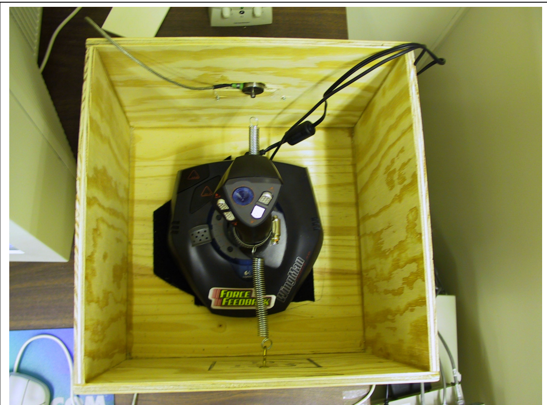
Figure 2. Top view of the joystick calibration experimental setup
