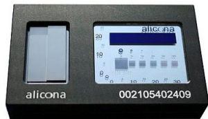
Lateral and Vertical Calibration Standard
