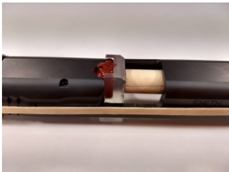
Casting of breech face surface
