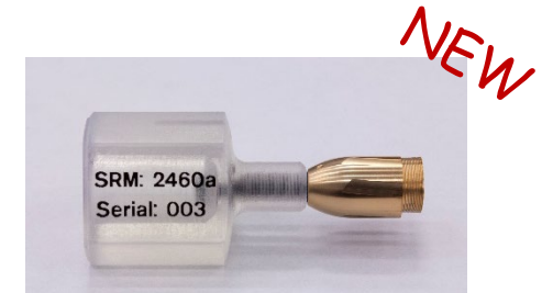
SRM 2460a Standard Bullet Replica
