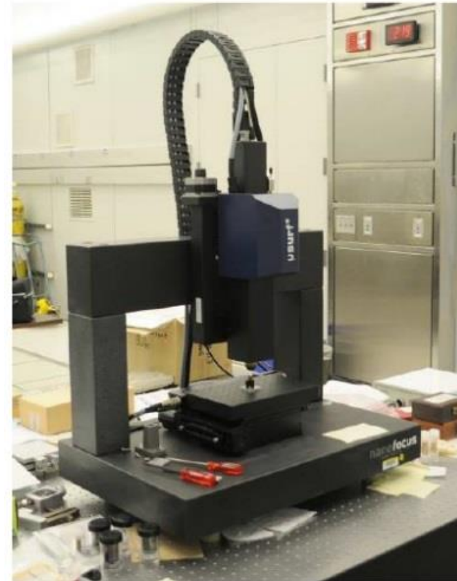
NanoFocus μsurf Disc-scanning confocal
