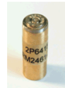
SRM 2460a Standard Bullet Replica
