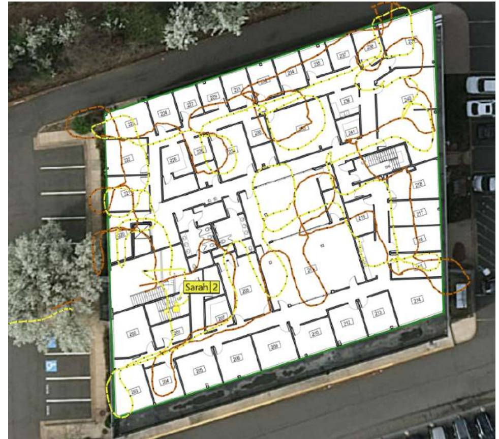
Relative Accuracy: 2D image of “ground-truth” (yellow) and a firefighter track on 3 rd floor
