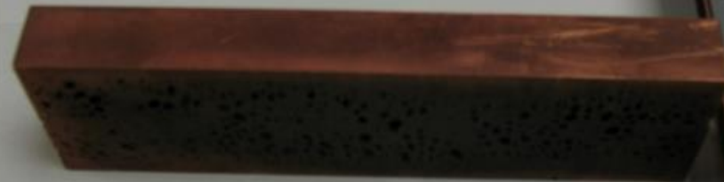
Edge view of center section of ingot, almost no porosity
