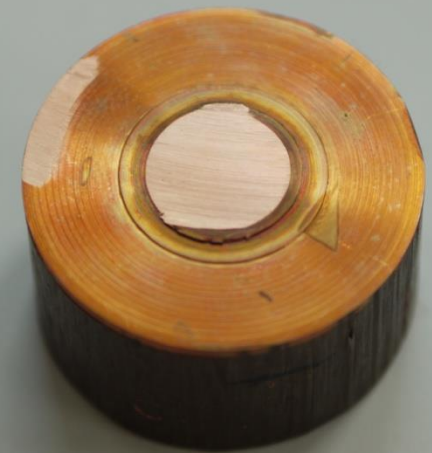
Section of Cu extrusion
