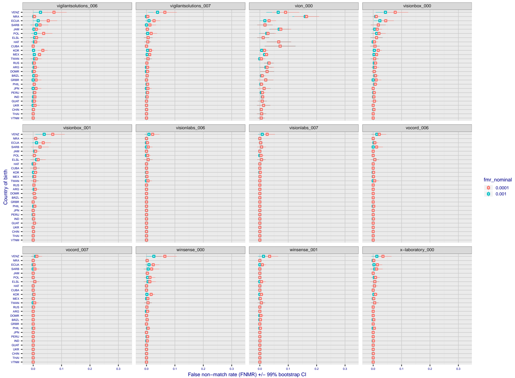
Figure 126: For the visa images, the dots show FNMR by country of birth for two globally set operating thresholds corresponding to FMR = \{0.001, 0.0001\} computed over all on the order of 10^{10} impostor scores. The FMR in each bin will vary also - see subsequent impostor heatmaps in sec. 3.6.1. The figures shows an order of magnitude variation in FNMR across country of birth; these effects are likely due quality variations, then demographics like age and race. The error rates in some cases are zero, and in others the DET is flat so the error rates at the two thresholds are identical. The lines span 1% and 99% of bootstrap replicated FNMR estimates.
