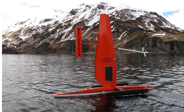
The Saildrone research platform is equipped with technologies to collect oceanographic data. Photo credit: Saildrone Inc.
