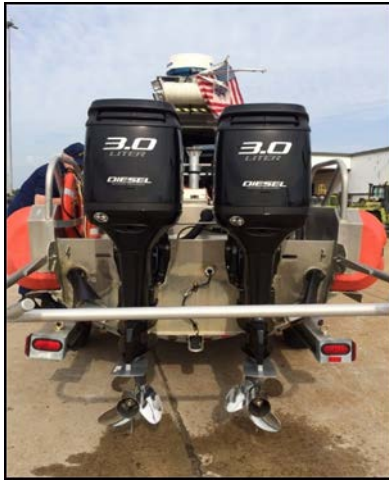
Two Mercury Marine 175HP spark-ignited diesel outboard engines installed on Training Center Yorktown's 25' Response Boat-Small for test and evaluation. USCG photo.
