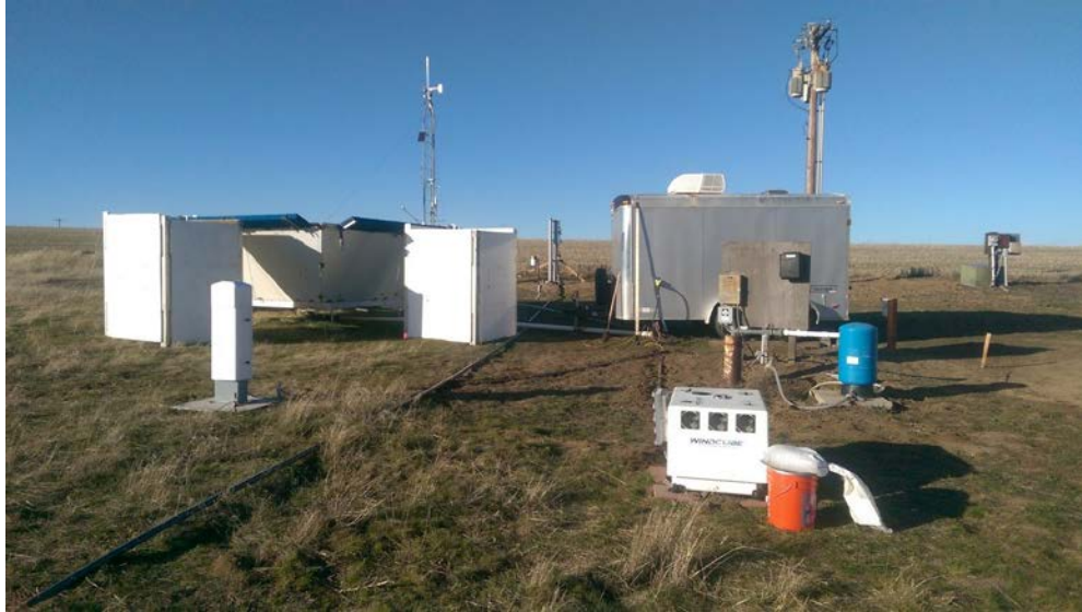
Instruments near the Wasco, Oregon site. (Front to back, left to right): Windcube lidar (deployed by CU/ATOC); ceilometer (deployed by University of Notre Dame); 915-Mhz wind profiling radar, trailer, and 10-meter tower with additional instruments (deployed by NOAA ESRL PSD). Photo courtesy of Justin Sharp.
