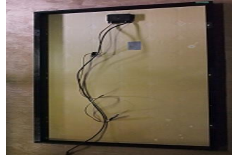
Yellowing in PET Backsheets observed in the field
