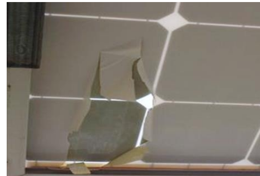
Cracking and delamination in 1s PVDF Backsheet
