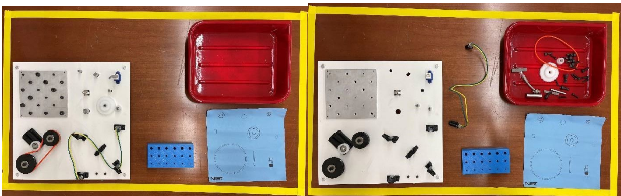
Figure 4: Subtask 2 – Disassembly. This subtask starts with a fully assembled task board (a). Completion results in a fully disassembled task board with all loose components placed in the tray. Note: Kit mat layout will change.
