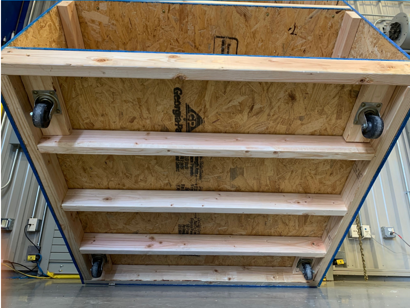
CABINET BASE UNDERSIDE
