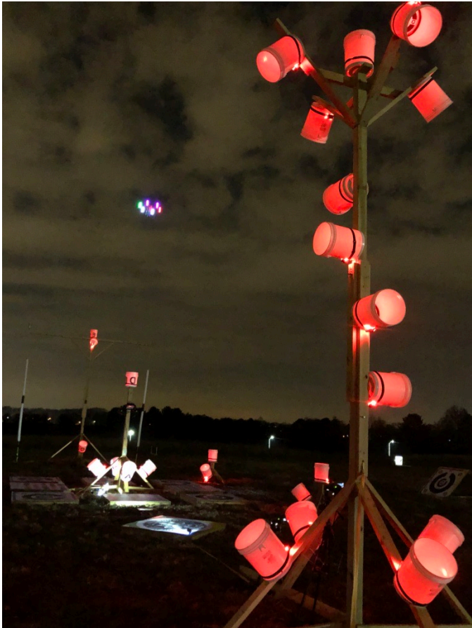
Position accuracy for range to target using lighted buckets (red or white)
