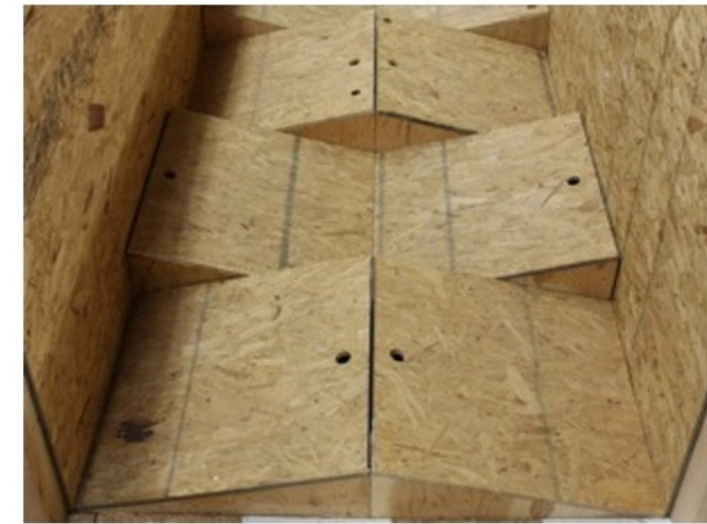
Crossing Ramps (E2826)
