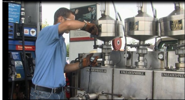
Figure 6 – Inspector Draining a Prover
