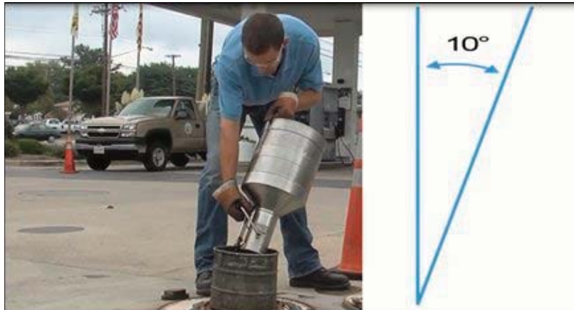
Figure 3 – Inspector Draining a Test Measure at a 10° to 15° Angle.
