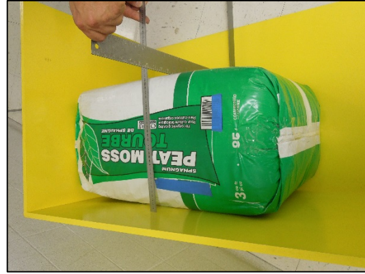
Figure 3-6. Width Measurement – The frame is rotated on its end to vertical so that the carpenter square does not compress the product.
