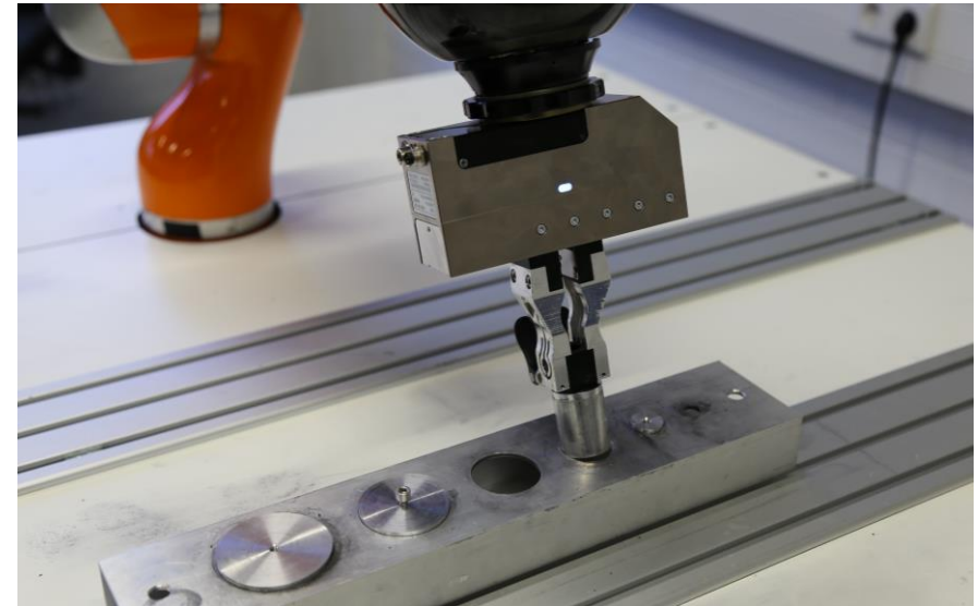
DLR Lightweight Robot with Adaptive Impedance control in peg-in-hole experiment
