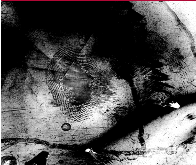
Conventional DFO fluorescence image, excitation wavelength 460 nm, Nikon D 200 in macro mode 2,8/60 , Type 23 Filter
