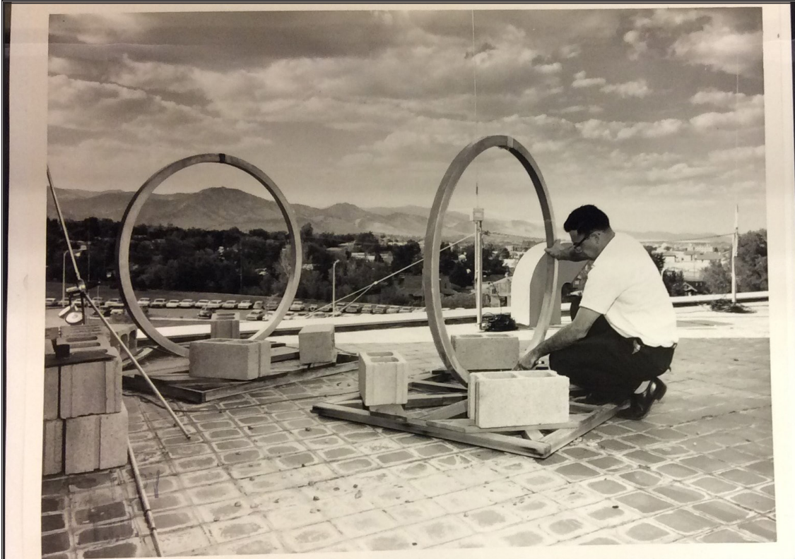
Figure 2.3: NIST physicist Lowell Fey makes an adjustment on the receiving antenna for phase lock control of WWV and WWVL, located at Fort Collins, of the Radio Building of the Boulder Laboratories, 1964. (courtesy of the National Archives at Denver).
