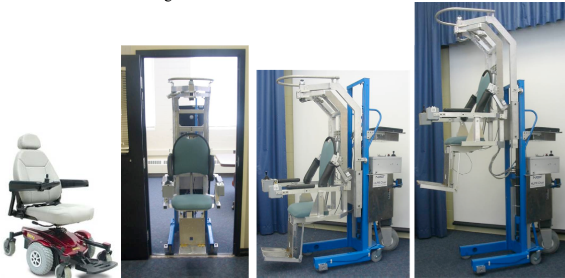
Figure 1: Typical powered chair (left) [courtesy Jazzy 1 ] and the HLPR Chair 1 prototype (right three photos). HLPR Chair is shown in the mobility (center photos) and the lift (left-most) configurations. Note the unique shape of HLPR Chair as compared to typical powered chairs.
