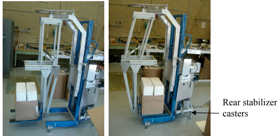
Figure 2. HLPR 1 prototype transitioned into an articulated forklift and shown in the (left) loading and (right) loaded-mobility configurations.
