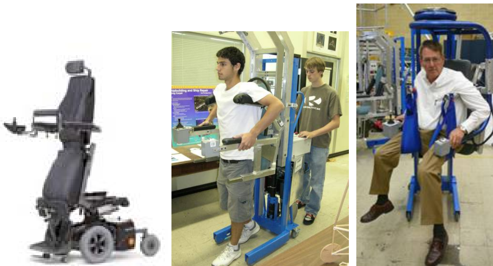
Figure 8. (left) Off-the-shelf standing type powered chair (courtesy Permobil), (center) HLPR Chair 1 in the patient rehabilitation configuration. The prototype is supporting a patient while they or a caregiver (behind HLPR) commands HLPR to move. (right) HLPR Chair 2 supports a patient with a sling ready for transfer to a seat, toilet or bed.
