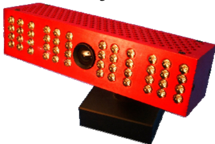
Figure 1 – CSEM SwissRanger2 3D Range Camera
