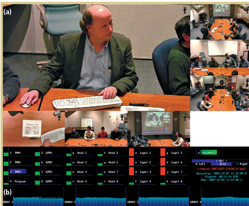
Figure 1. The US National Institute of Standards and Technology (NIST) Meeting Room Data Collection Laboratory in operation, using the NIST Data Flow System (NDFS) for data transport, synchronization, and storage, as seen at the review station: (a) one pan-tilt high-definition camera (upper left) can follow a presenter, while the other six high-definition cameras show whiteboards, written materials, projector displays, and the other meeting participants; (b) the system displays input levels for 24 individual microphones and four high-resolution NIST Mark-III 64-channel microphone arrays.
