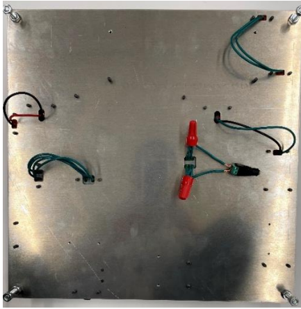
Underside of task board showing wire connections
