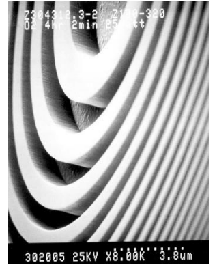
Fresnel Zone Plate , manufactured using ebeam lithography + etching
