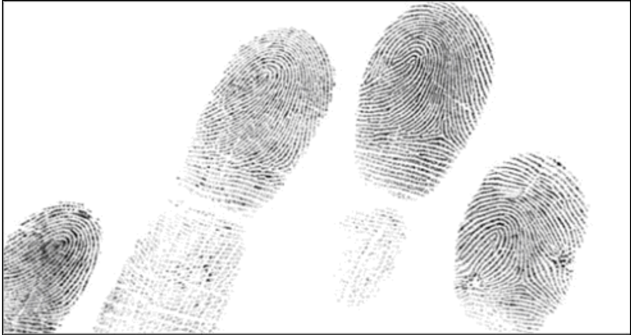
Figure 2. Sample unsegmented 4-finger livescan slap image. Unsegmented images were not used in FpVTE: see Figure 3 for the corresponding segmented images. Note that part of the little finger was not included in the slap image: incomplete fingerprints such as this can sometimes occur with any finger in slap images, especially for images from paper sources or from livescans with smaller platens.
