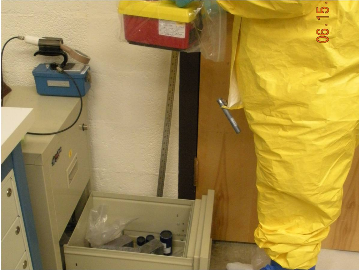
Figure A4. Fire-proof, radioactive source storage cabinet (shown during entry to the contaminated lab). Other glass-bottled source and lead bricks can be seen in the drawer.
