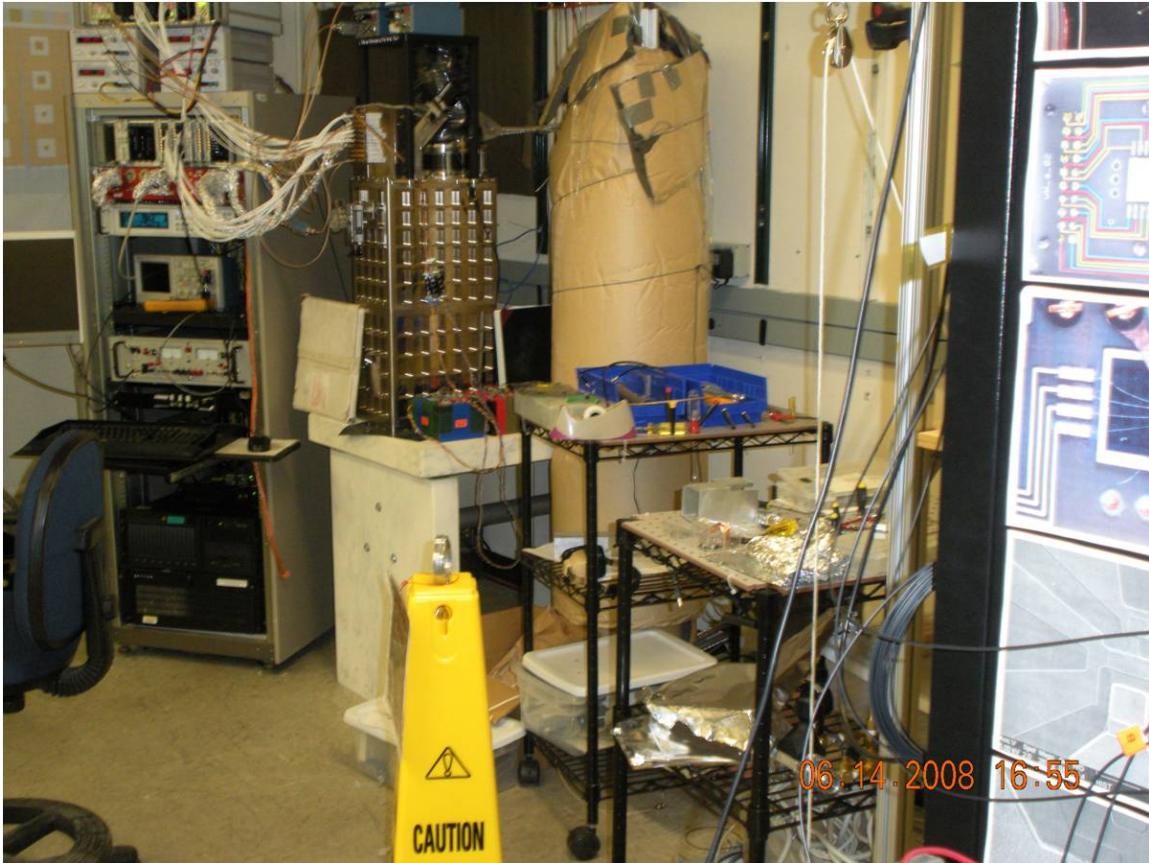
Figure A1. Laboratory 2124 showing the contaminated detector area. The detector is the rectangular device on the white bench in the left-center of the picture. The control computer is located in the electronics rack shown in the left side of the picture. The source position is located between the detector and the electronics rack and is not visible in this photograph.
