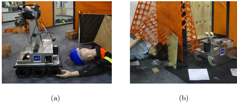
Fig. 1. On the left the six wheels platform, designed to enter the yellow and orange arenas. On the right the tracked platform, designed to enter all the arenas.
