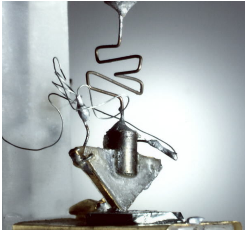
First Transistor, 1947 William Shockley, John Bardeen, and Walter Brattain
