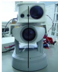
Fig.3 integrated sensor (lower: visual sensor, upper: laser distance meter )
