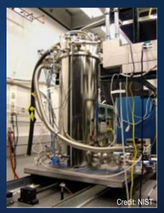
NIST Primary optical watt radiometer (POWR)
