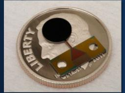
Credit: Nathan Tomlin, NIST cryogenic fiber optic radiometer (NIST-on-a-CHIP)
