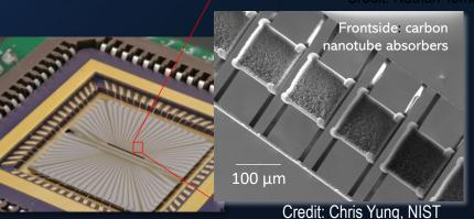
Microbolometer Array for Far-Infrared
