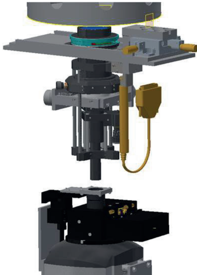
Figure 4.17: Inventor drawing of new imaging system and mounting configuration, designed by Jonas Keller.
