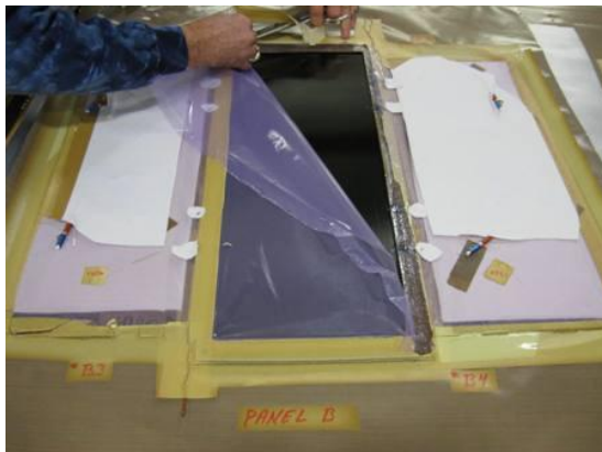
Cured laminate being un-bagged
