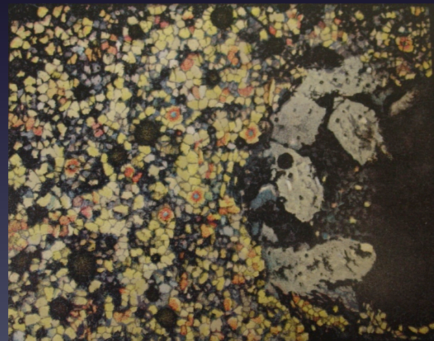
Tricalcium silicate (gray), along with dicalcium silicate crossed Nichols, 190x
