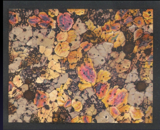
Thin section of dicalcium silicate, crossed Nichols, 90x
