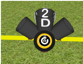
RIGHT ANGLED BUCKET INTERIOR BOTTOM ORIENTED TO READ LETTER UPRIGHT WHEN MOUNTED
