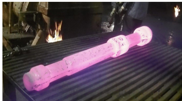
Figure 4. Forged Ferrium M54 Hook Shank
