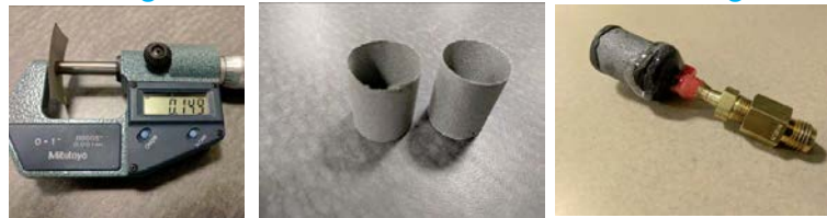
Conformal HeX (steel) Weight Minimization, Thickness & Leakage
