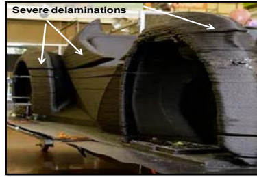
3D Printed Shelby Car Minimize Delamination
