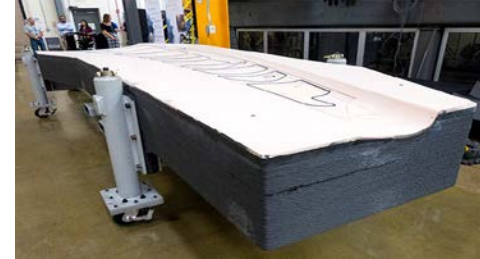
Wing (Thermoplastic-PPS) Delamination/CTE
