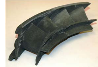
Ceramic Part (Binder Jet) PIP & Voids
