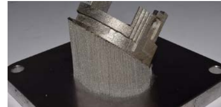
Mount Ring (Inconel 718) Roughness, Warpage, Base Plate & Support Design
