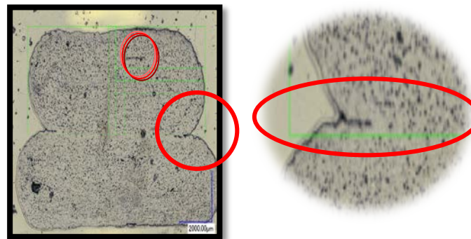
Cracks within/between Beads
