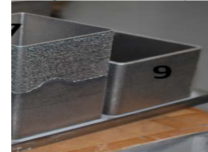
Mount Ring (Inconel 718) Roughness, Warpage, Base Plate & Support Design
