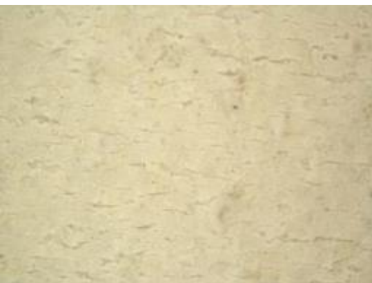
TPT-3: Cracking observed for the air side (PVF) is shown in a microscopy image of the surface.
