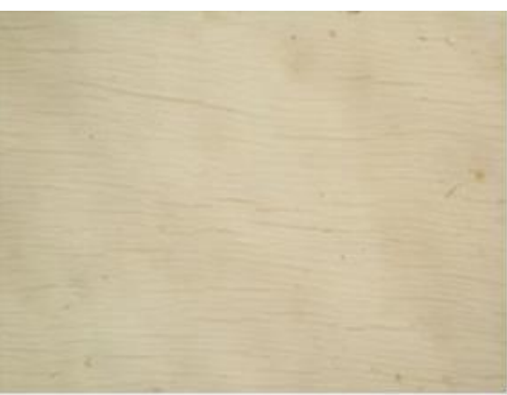
PA: Cracking observed for the air side (PA) is shown in a microscopy image of the surface.
