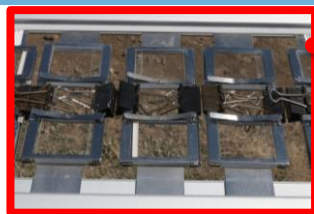
Unbacked transparent coupon specimen may reach very different temperatures than PV modules (TG5 Study 1).
