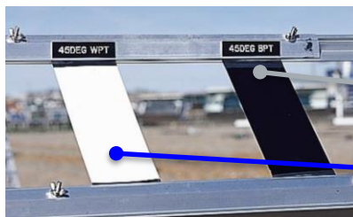
White panel, black panel, other... temperature is still a concern in natural weathering. Feil, Proc. ASTM G03 Work., 2019.
