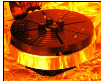
New adjustable mechanical chuck holds wafer pieces without using a vacuum. This design allows a uniform layer of resist to be applied while reducing the risk of rupturing fragile nitride membranes.
