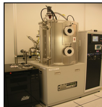
A second vacuum E-beam evaporator is now available in the NanoFab cleanroom.
