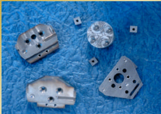
NIST micromechanically machined STM components
