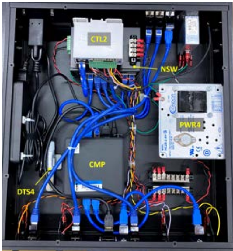
Figure 4.24: SPU Power Control Tray
