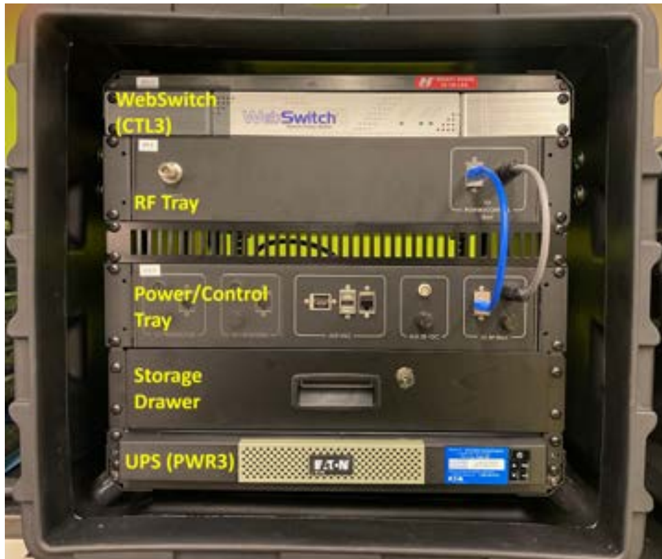
Figure 4.23: SPU Assembly (9U)
