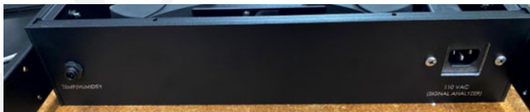
Figure 4.29: SPU RF Tray Rear Panel
