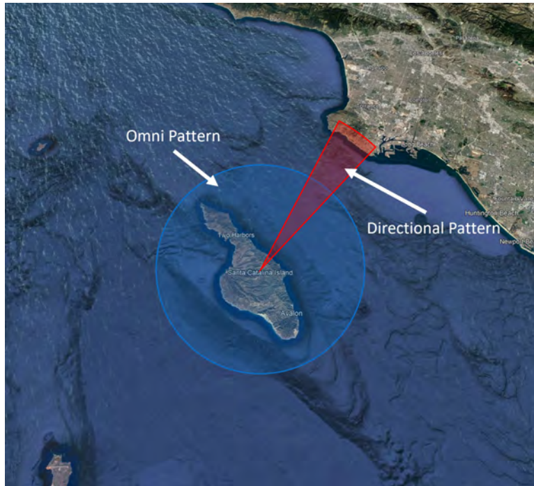
Figure 6.6: Example omni-directional and directional antenna patterns with relative gain located on Catalina Island.
