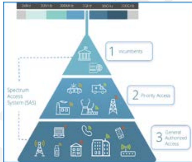
Figure 1.2: FCC's three-tiered access for CBRS. Reference: https://ongoalliance.org/the-technology-behind-spectrum-sharing-the-spectrum-access-system/
