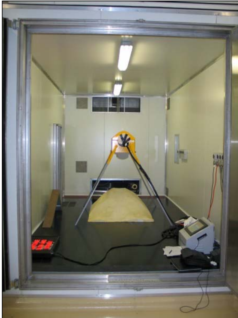
Custom-mounted LVS in environmental test chamber, NMI, Sydney, Australia
