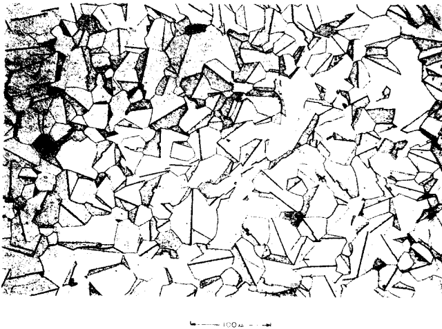
Figure 1. Photomicrograph of a polished and etched section of a metal oxide varistor.
