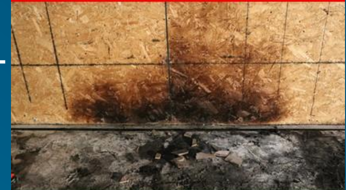
Significant thermal damage to OSB
