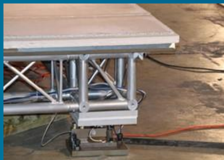
Uninsulated Load Cell
