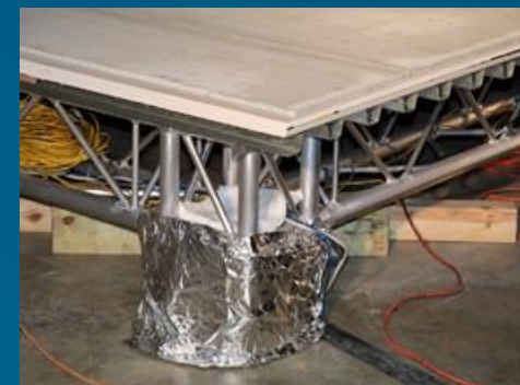
Insulated Load Cell
