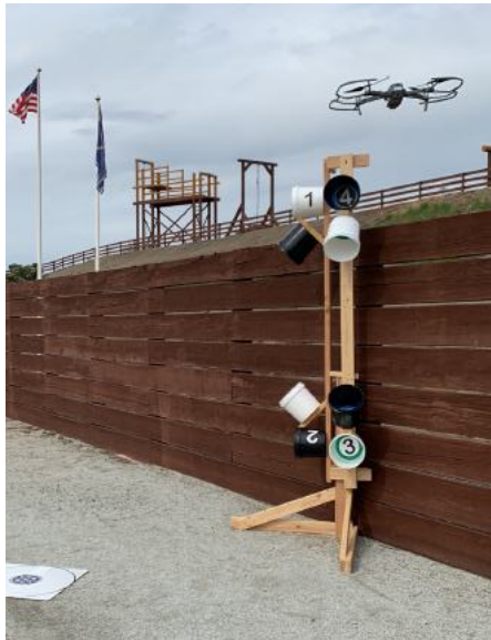
The WALL test shown with alternating pairs of white and black buckets to increase the need for exposure control.
